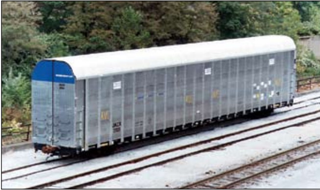
Figure 2a. Aluminum Vehicle Carrier (AVC). (Photo courtesy of Johnson America Corp.)
