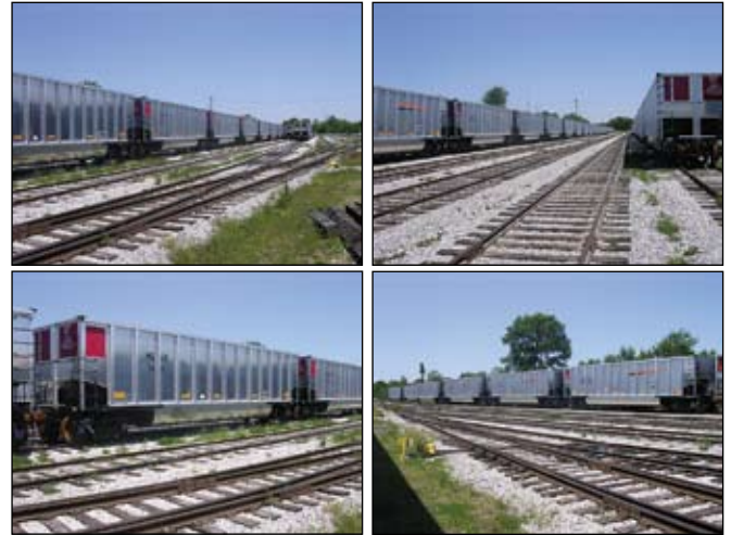
Figure 1. Aluminum intensive open-top hopper cars. (Photos courtesy of Freight Car of America)
