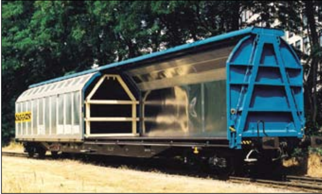
Figure 2b. High capacity railcar with sliding aluminum sidewall. (Photo © Alstom Transport)
