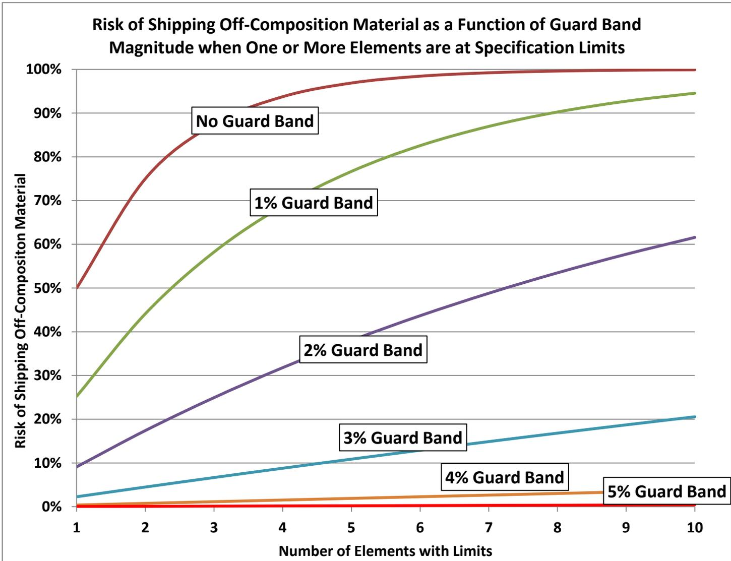
*Figure 6. Probability a cast is off-composition for product with guard bands between 0 % and 5 % of the nominal concentration for a sample assuming a 3 % relative uncertainty in analysis.*
