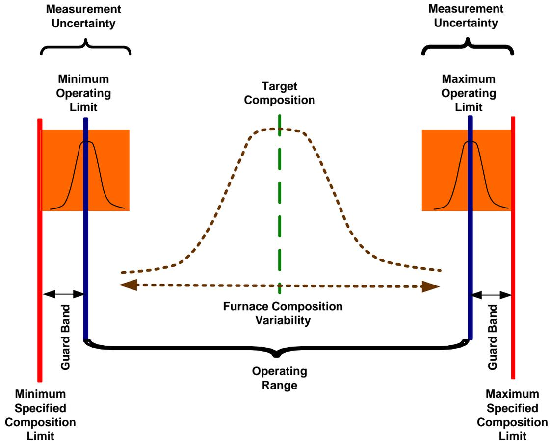
**Figure 3 illustrates the case where the specified composition range is wide enough to accommodate both the furnace composition variability and guard bands to account for Spark-AES test method uncertainty. This is the best case scenario for reliably producing product that meets specified composition limits.**
