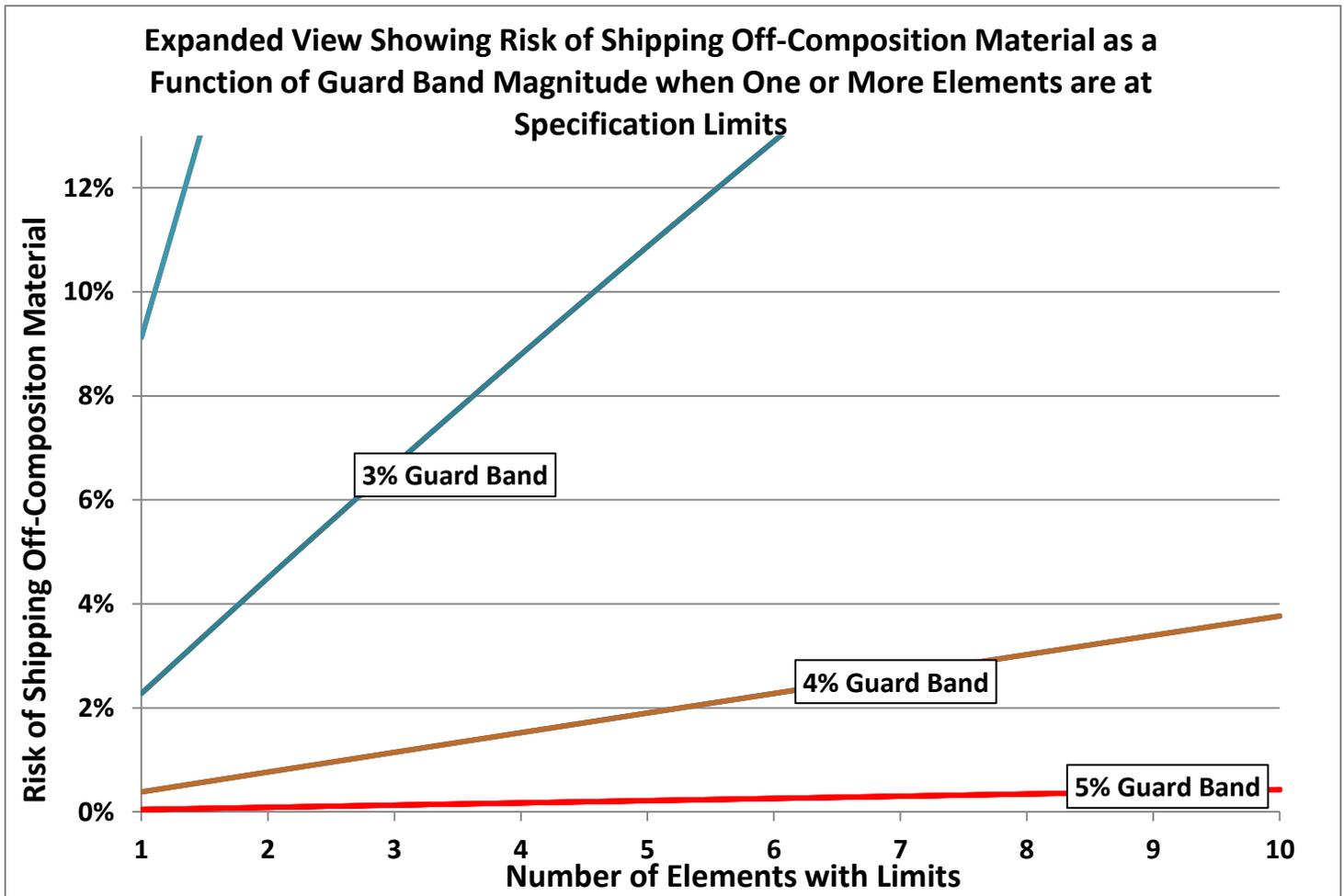
*Figure 7. Expanded scale - Probability a cast is off-composition for product with guard bands between 3 % and 5 % of the nominal concentration for a sample assuming a 3 % relative uncertainty in analysis.*
