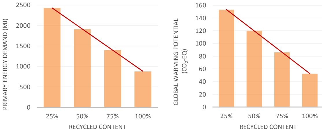
Figure 6. Sensitivity of PED and GWP towards the recycled content (recycled content scenario)
