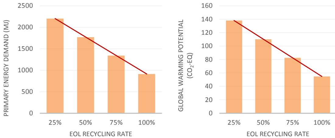
Figure 5. Sensitivity of PED and GWP towards the end-of-life recycling rate (avoided burden scenario)
