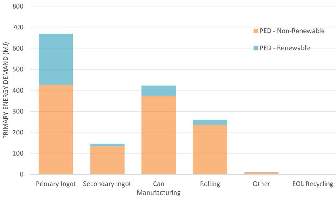
Figure 4. Breakdown of primary energy demand (recycled content scenario)
