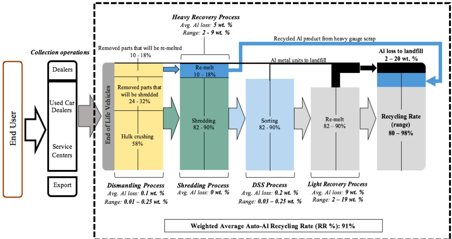
Figure 4: Process material flow analysis for automotive aluminum.
