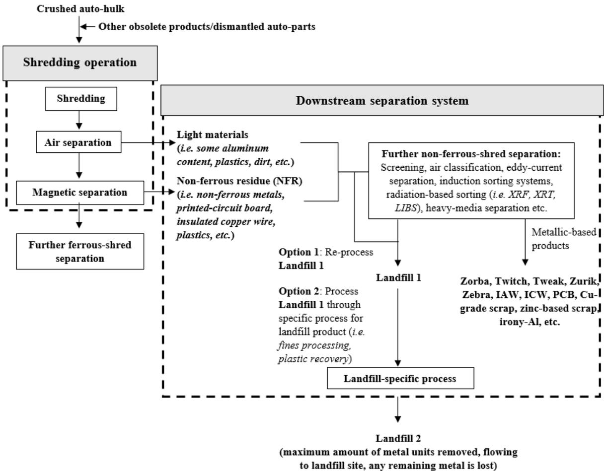
**Figure 2: Shredding operation and downstream separation system definitions.**
