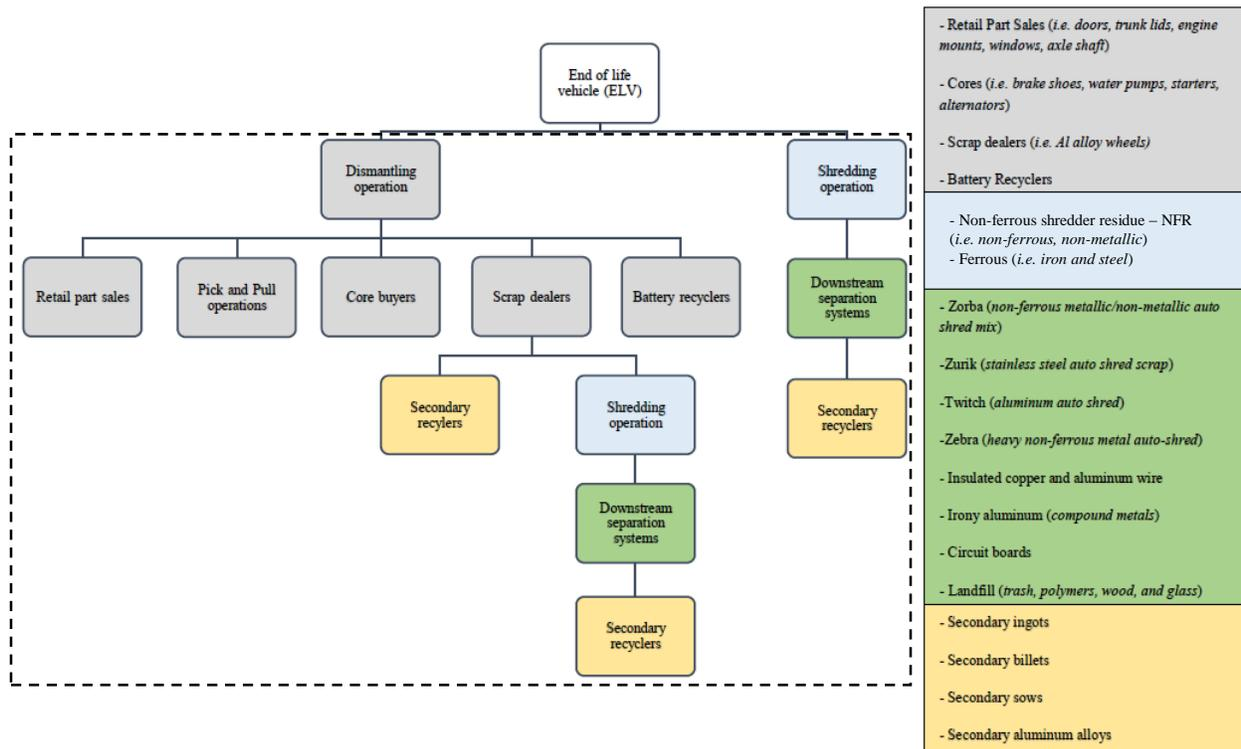
Figure 1: End-of-life vehicle process flows with process-specific product outputs.
