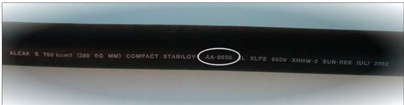
Photo 2. Legend on commercially available AA-8000 conductor
